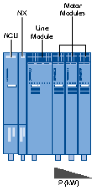
Figure 2-7 NX between NCU and Line Module
