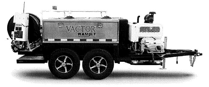
The Ramjet trailer & skid-mounted jetters are the perfect machines for fast, safe response to sewer blockages as well as regular preventative line maintenance. Our line of reliable, high-pressure water jetters are specially designed for cleaning municipal sewer, drain and pipe lines as well as culverts at low water volume. These units are ideal for cost effective maintenance and emergency response in tight, confined environments.
